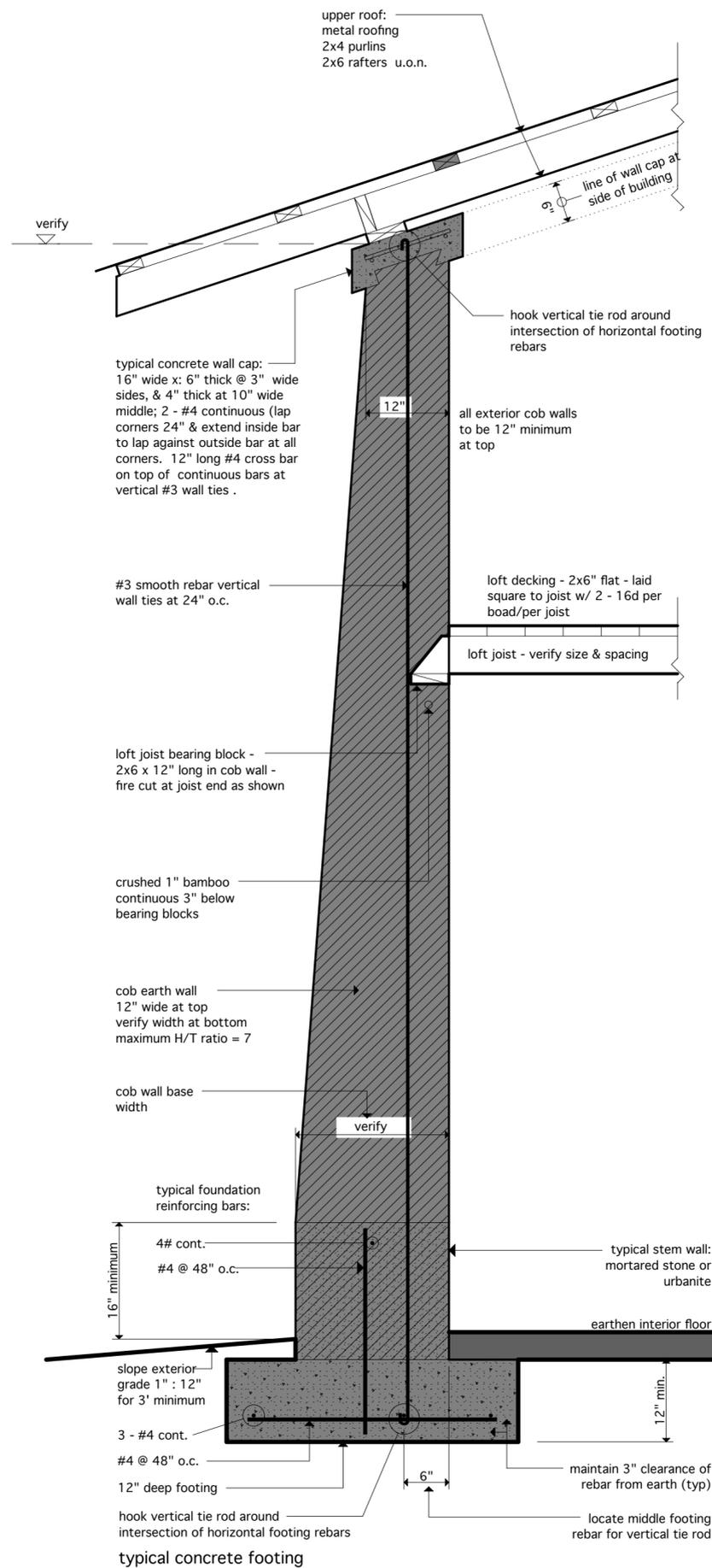
**WALL WITH UPPER LOFT AND CONCRETE BOND BEAM**
