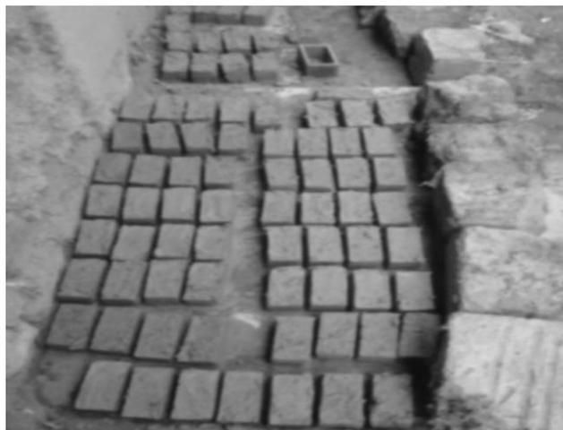
**Fig. 3. Recycled sugarcane fiber waste bricks**
