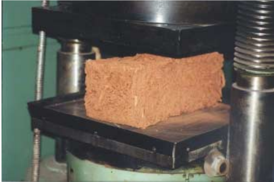
Photo 1. First load deflection test
