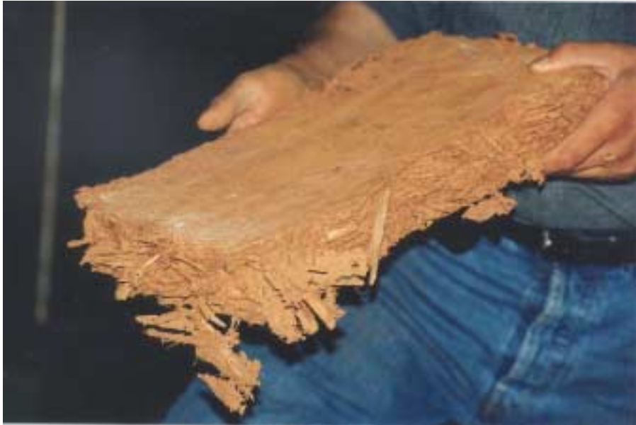
Photo3. Stable light clay plate after the load deflection test.
