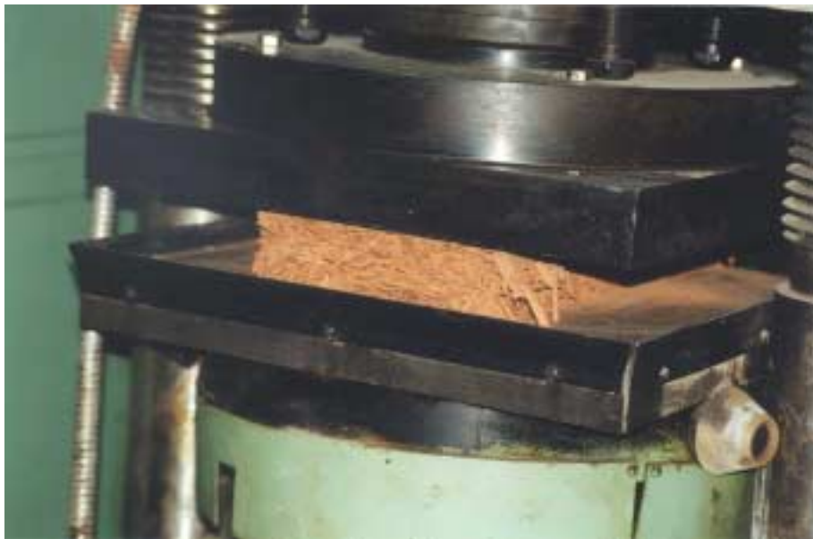
Photo 2. Light clay is hardly disintegratable in high compression
