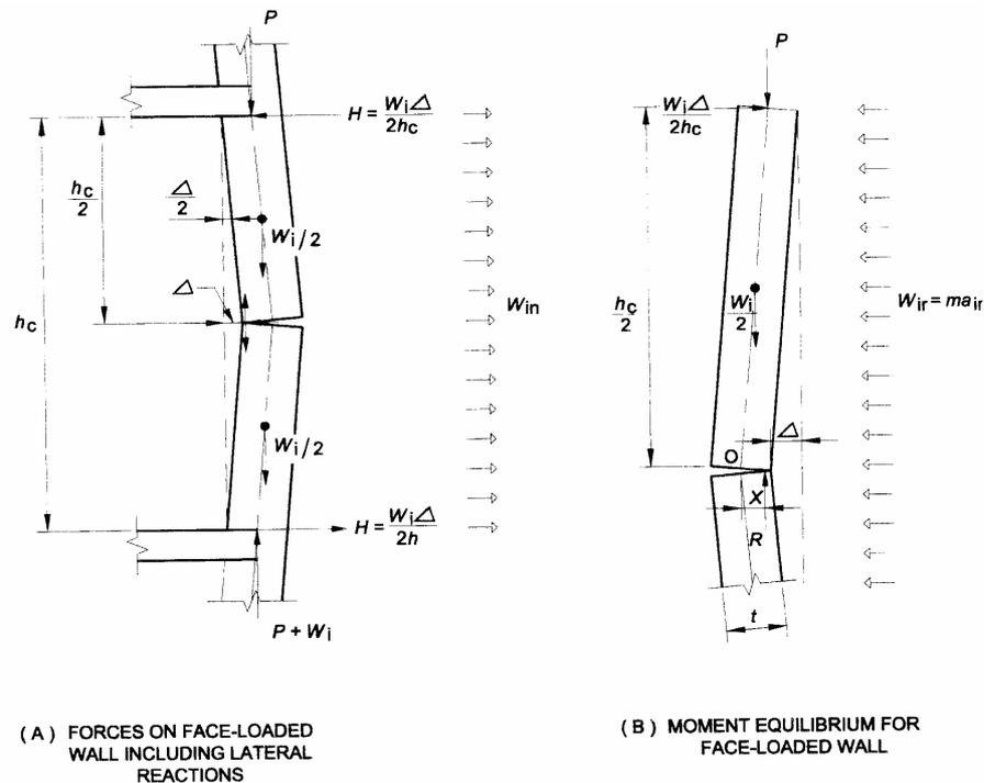
**Figure 23** Moment equilibrium parameters for determining the out-of-plane performance of unreinforced walls in low earthquake zones
