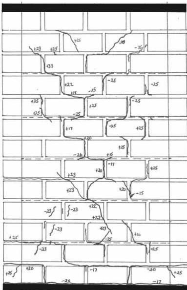
**Figure 19** Crack pattern of the adobe wall showing the load progression
