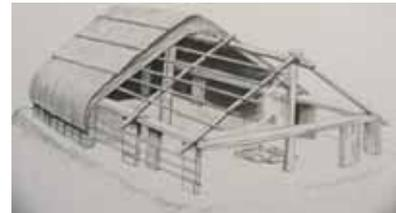
**Figure 4** Early Maori housing – low earthquake vulnerability
