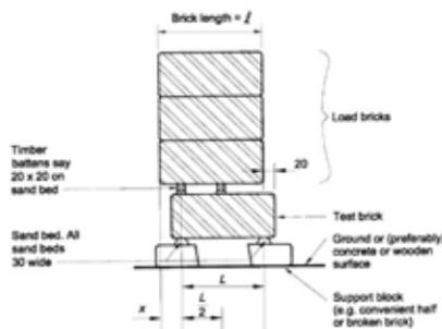
**Figure 12** Modulus of Rupture Test
