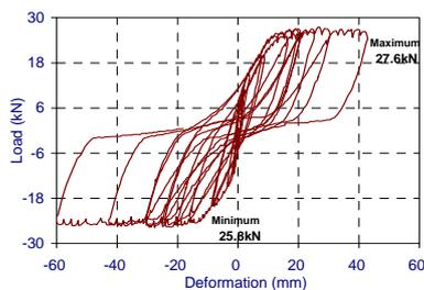
**Figure 18** Cyclic load performance of 1.2m x 1.8m adobe wall
