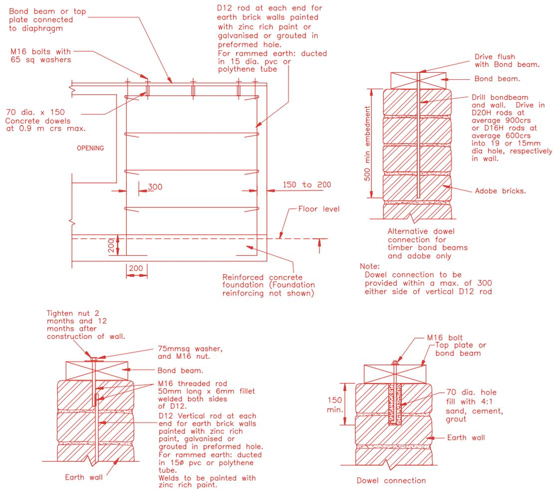
**Figure 15** Typical reinforced wall detail from NZS4299 – Polypropylene geogrid is also used horizontally
