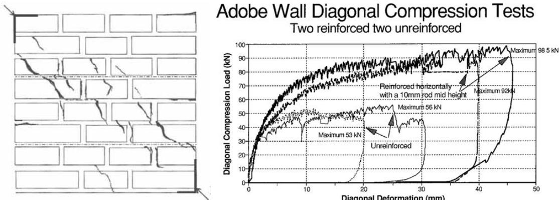
**Figure 16** Diagonal compression tests of adobe showing the crack pattern and results
