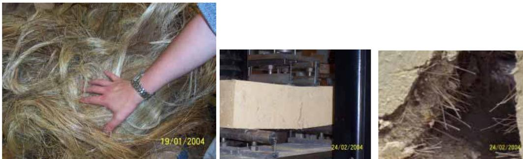
**Figure 21** Fibre from New Zealand flax, MOR test of fibre reinforced soil-cement beams
