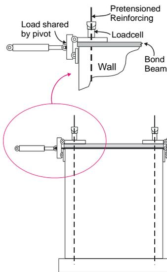
**Figure 17** Load configuration for in-plane panel tests
