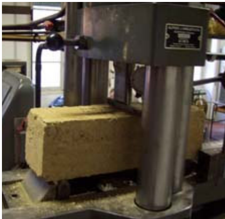
Figure 7: Test of compression (on the left); Diagram of tension – deformation of the earth A (on the right).
