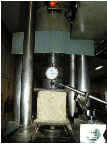
Figure 7: Test of compression (on the left); Diagram of tension – deformation of the earth A (on the right).
