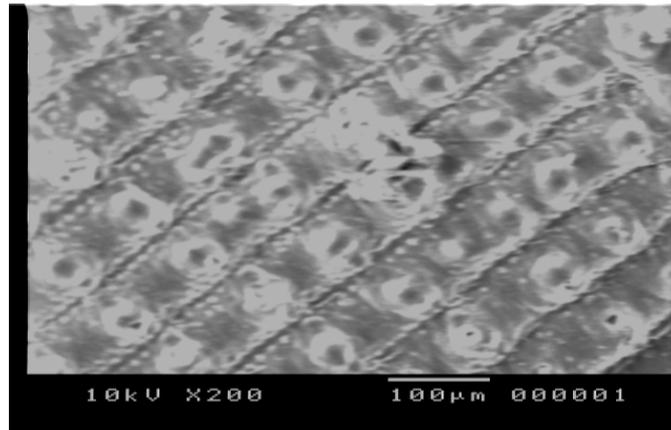
FIGURE 2- SEM MICROGRAPH OF ALKALI TREATED RICE HUSKS 4% NaOH
