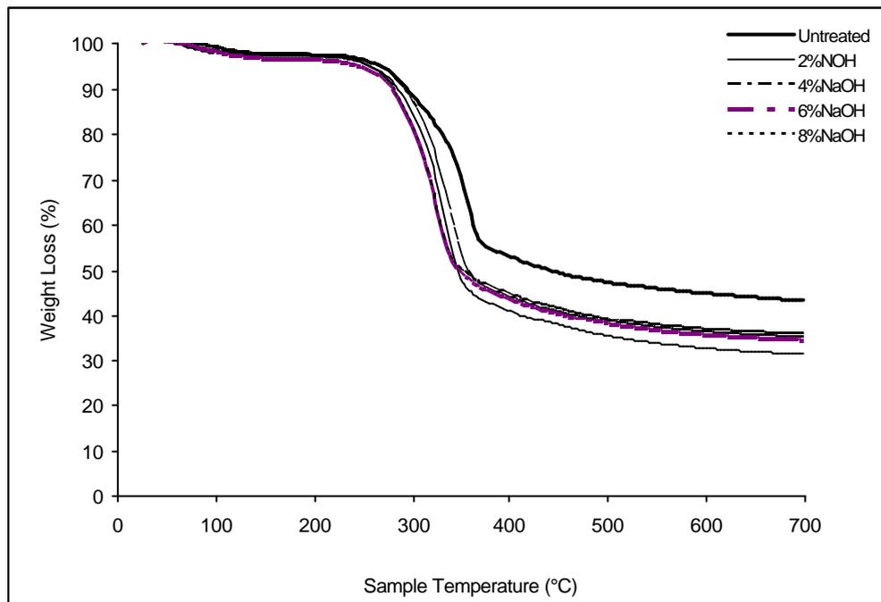
**FIGURE 7-** TGA THERMOGRAMS OF UNTREATED AND NaOH TREATED RICE HUSKS
