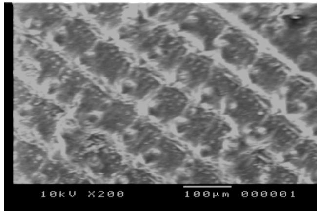
**FIGURE 1-** SEM MICROGRAPH OF ALKALI TREATED RICE HUSKS 2% NaOH
