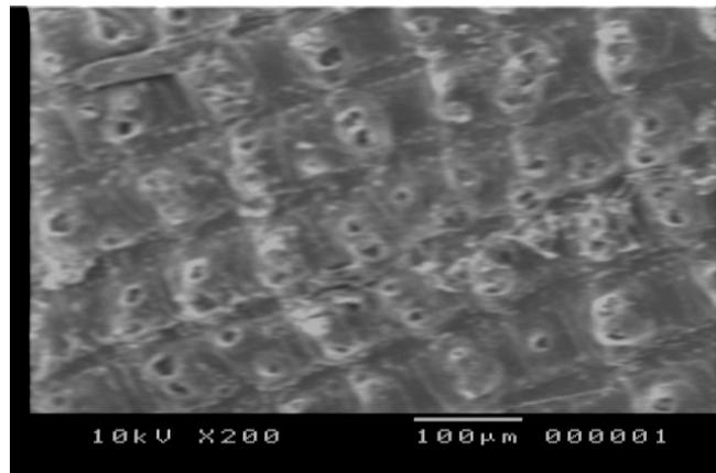
FIGURE 3- SEM MICROGRAPH OF ALKALI TREATED RICE HUSKS 6% NaOH
