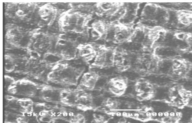
FIGURE 4- SEM MICROGRAPH OF ALKALI TREATED RICE HUSKS 8% NaOH
