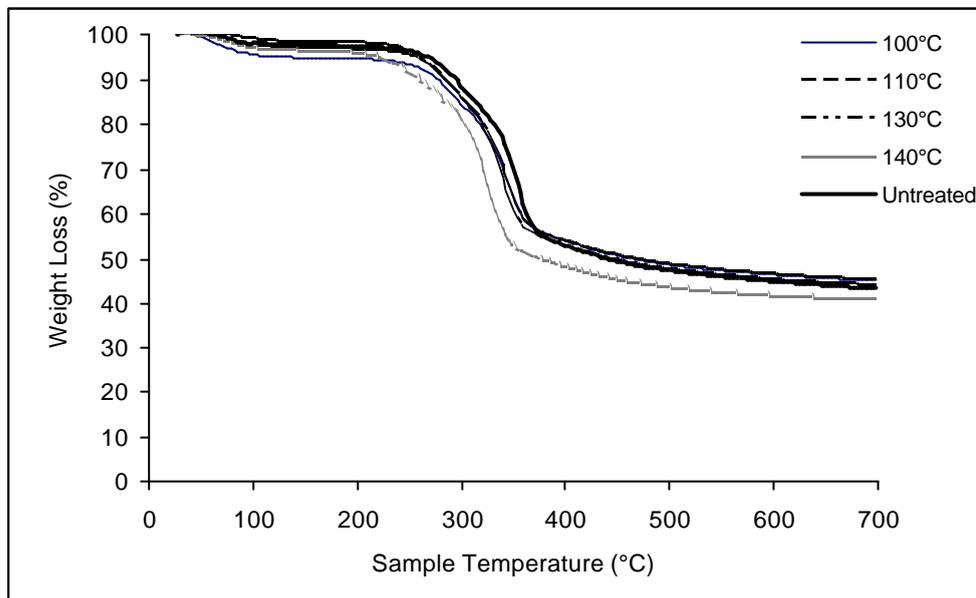
**FIGURE 8-** TGA THERMOGRAMS OF UNTREATED AND STEAM CURED RICE HUSKS
