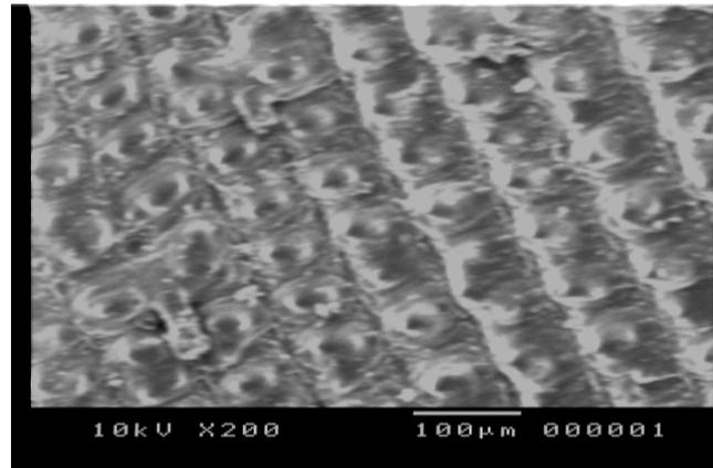
FIGURE 5- SEM MICROGRAPH OF STEAM TREATED RICE HUSKS 130°C
