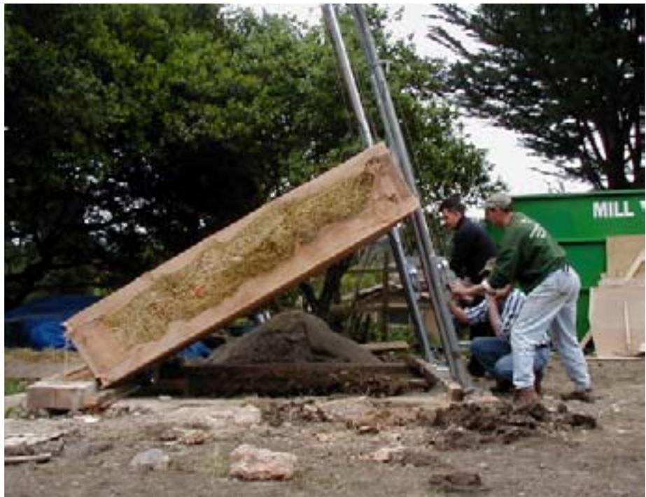
*Out-of-plane load test*
